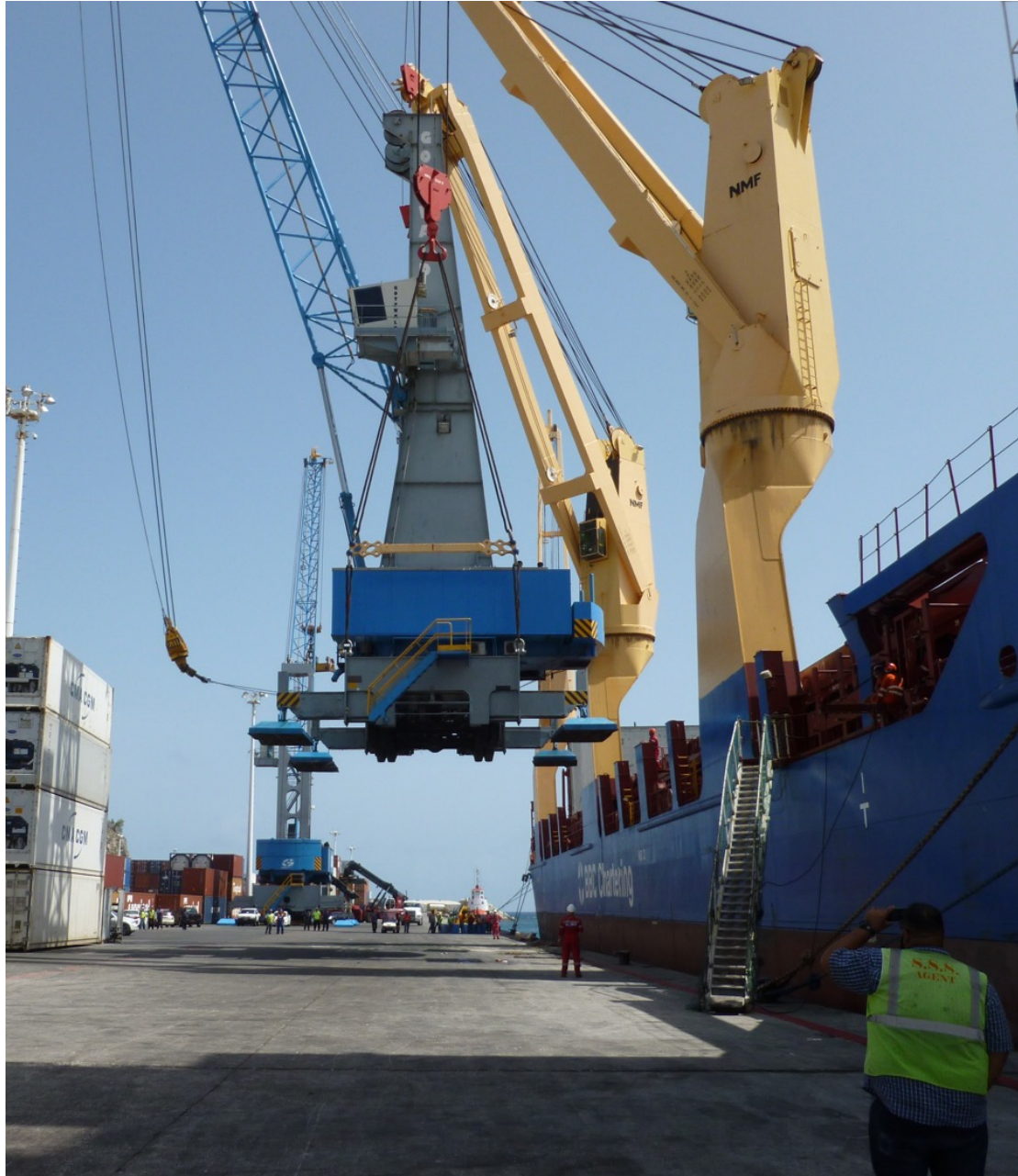
PHOTO CUTLINE: Gottwald crane HMK 260E being loaded on the Cargo Vessel BBC Congo.
